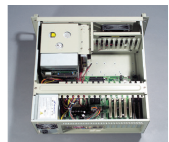
Motherboard can fit in 450 mm (17.7") depth
